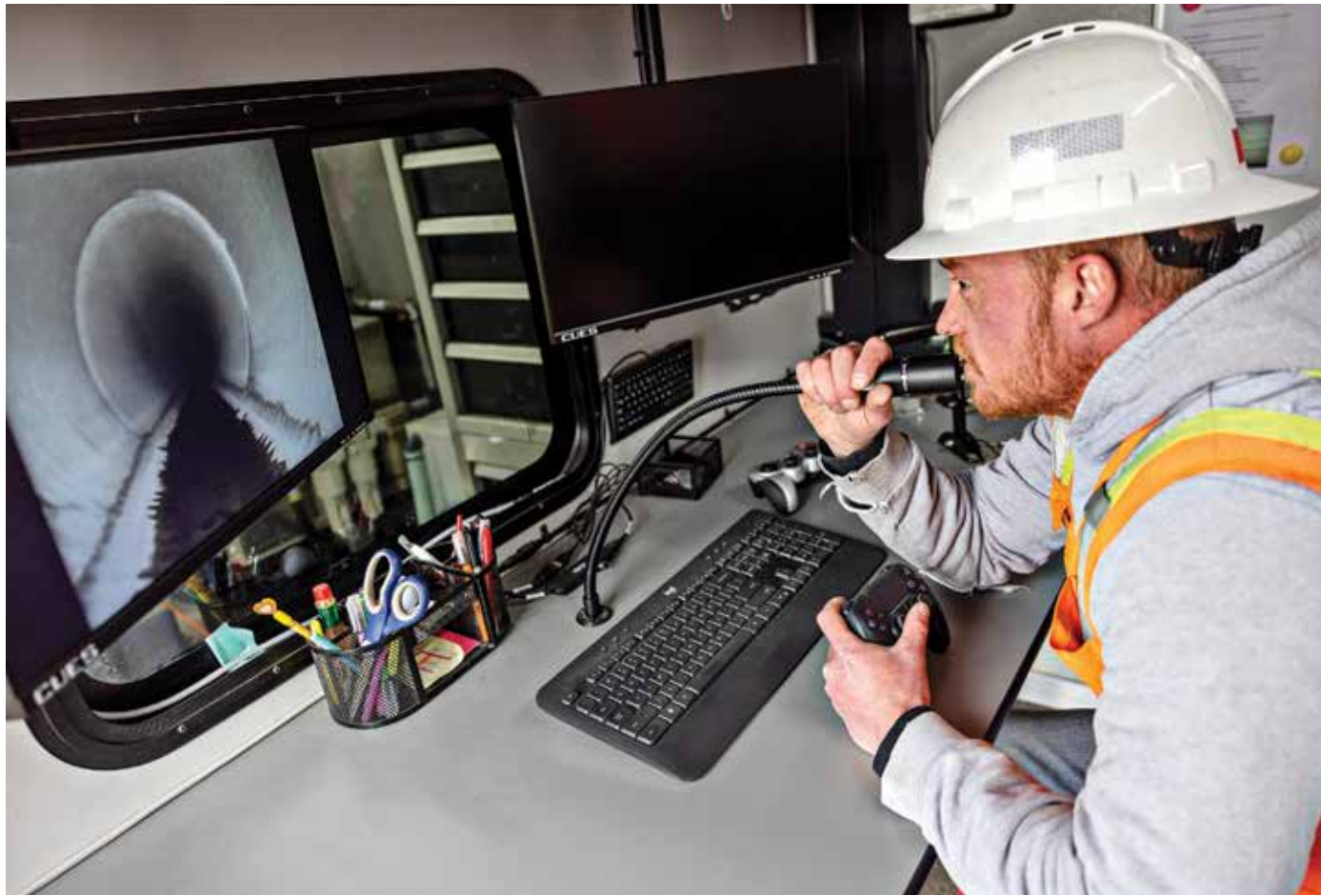
» Christopher Coots reviews footage from a pipeline inspection.
